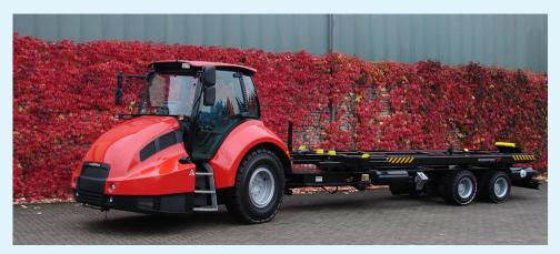
Load carrier Swopper XT for relocation of containers
