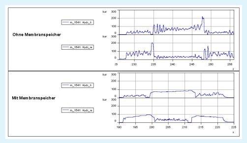
Comparison of the pressure surges in original state (above) and with installed hydraulic system (below)
